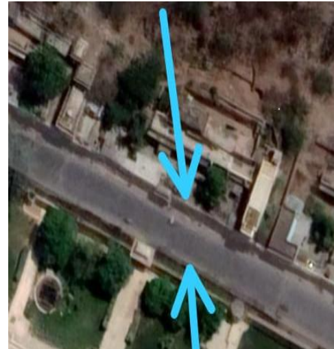
Fig. 1: Median is missing in the narrow stretch of the road
