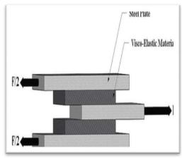
Fig.no.2: Viscoelastic Dampers
