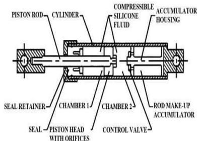
Fig.no.1: Viscous Damper
