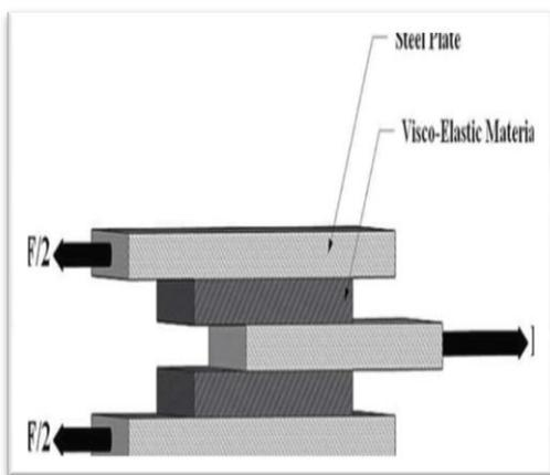
Fig.no.2: Viscoelastic Dampers
