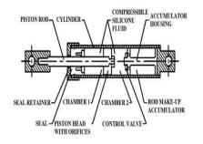
Fig.no.1: Viscous Damper
