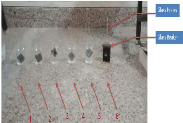
Fig 1: Corrosion Process with various environments (Contact hr. range: 72 hrs., 140hrs, 240 hrs.). (Chemical used here: H 2 SO 4 , KOH, NaOH, HNO 3 , HCl, Chromic Acid)
