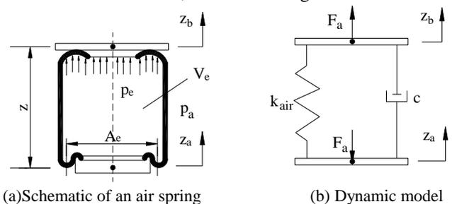
Figure 1: Dynamic model of an air suspension system
