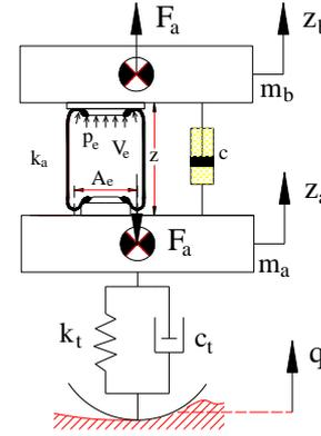
Figure 2: quarter-vehicle dynamic model of a heavy truck with two degrees of freedom
