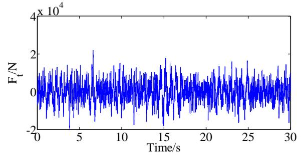
Figure 5: The vertical dynamic tire loads acting on road surface with Case 3
