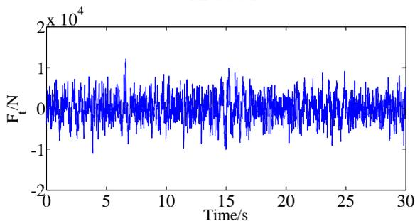
Figure 4: The vertical dynamic tire loads acting on road surface with Case 2
