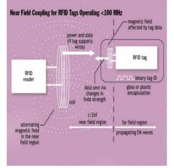
Fig. 1. RFID working Principle
