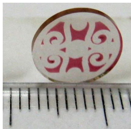
Fig. 2. HAuCl 4 /PMMA sample obtained by bulk polymerization. Color parts are obtained by UV 20 min irradiation by XeCl laser through the mask and subsequent annealing over 3min at 160 °C. These colored domains contain Au nanoparticles (for details see [3]).
