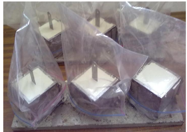
Fig 1. Set of 6 out of 18 cement paste specimens with stainless steel sheets to form artificial cracks
