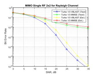
Fig. 10Detector Performance in MIMO-OFDM System Based on Single-RF.
