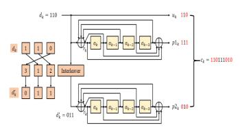
Fig. 4 Turbo Encoder (1,33/37)Rate 1/3.
