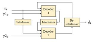
Fig. 5 Turbo Decoder Rate 1/3.
