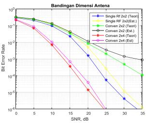
Fig.11 Antenna Comparison in MIMO-OFDM System Using Turbo Code
