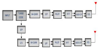
Fig. 6 Block Diagram of MIMO-OFDM System Transmitter.
