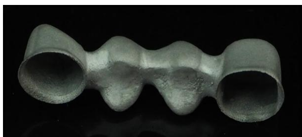
Fig. 6. The prosthetic bridges after selective laser melting before (a) and after (b) sand-blasting. The applied parameters: laser power at building the contour 50 W, laser power at filling the contour 75 W, the spot size of the laser 0.13 mm, layer thickness 25 \mu m, oxygen level inside the chamber 0.2%, argon as technical atmosphere, the temperature of base plate 200°. The base plate was made of technical titanium.
