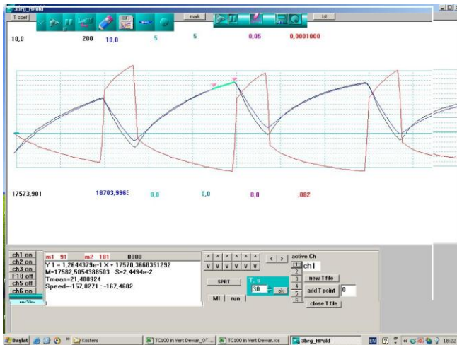
Fig.2. Simultaneous records of the resistance variations of a platinum resistance thermometer (PRT) and of two thermistors Th-1 and Th-2, which are located symmetrically relative to the PRT on the surface of the gauge block. During the current modulation cycle in the PRT, its current for \frac{1}{4} of the modulation period is kept at the level of 5mA and \frac{3}{4} of the period is kept at 1mA. The sensitivities of the thermistors are, practically, equal. Two cursors (shown by triangles) define the averaging time for the mean values of temperature quantities. (See text for other details).
