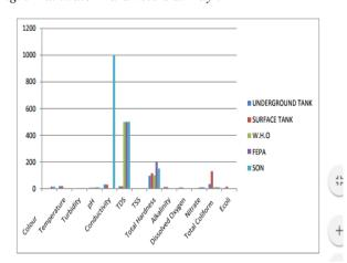
Fig. 8 Rainwater Parameters at Day 14
