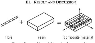
Fig-1: Composition of fibre-plastic composites
