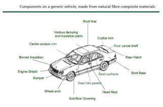
Fig-2: Components on a car, made from NFC material
