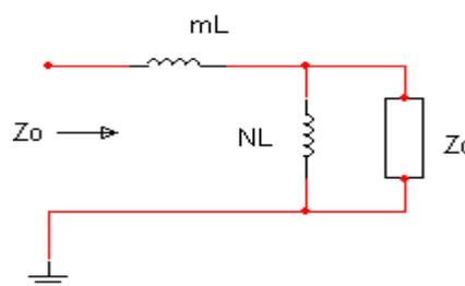
**Fig. 4** - A L-L single cell closed by its characteristic impedance  $Z_0$
