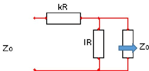
**Fig.6** -  $kR$ - $lR$  single cell with the characteristic impedance  $Z_0$ .
