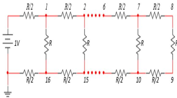
**Fig.11** Double resistive LN, non matched at its end with  $Z_0$
