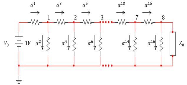
**Fig. 10** – Infinite discrete resistive LN: the currents across the branches of the LN are indicate
