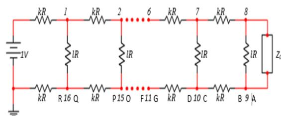
**Fig.15:** Resistive LN closed with the Characteristic impedance  $Z_0$  with longitudinal resistor value equal to  $kR$  and transversal resistor values equal to  $lR$
