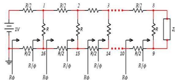
**Fig.14:** Double resistive LN matched with  $Z_0$
