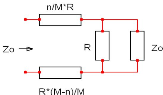
**Fig.16:** Dual ladder network made by longitudinal impedances whose sum is equal to R
