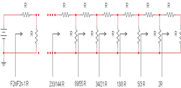
**Fig.8**—Resistive LN not closed with its characteristic impedance  $Z_0$ : impedance values in the indicated points. All the impedances are considered towards the right as indicated by arrows.
