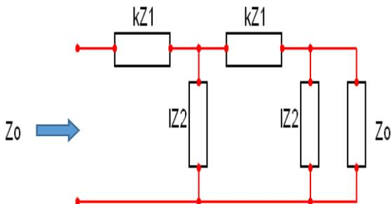
**Fig. 2-b)** Two cells of a ladder network terminated by the characteristic impedance  $Z_0$ .
