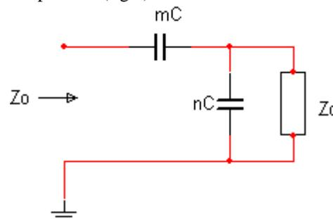
**Fig.5:**A C-C single cell closed on its characteristic impedance  $Z_0$
