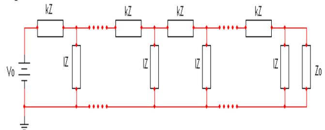
Fig.1 - Ladder network with impedances  $kZ$  and  $lZ$
