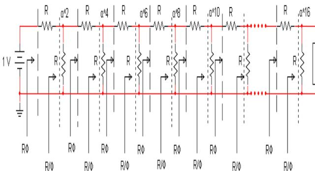
**Fig. 9**–Infinite discrete resistive LN: the voltages and the impedances along the line are indicated.
