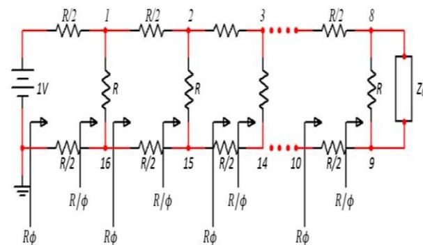
**Fig.12:** Double resistive LN matched with  $Z_0$
