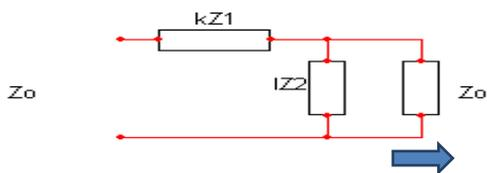
**Fig. 2-a)** Single cell of a ladder network terminated by the characteristic impedance  $Z_0$ .
