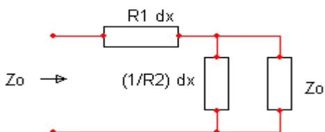
**Fig.3** Single cell for a continuous transmission line made by infinitesimal longitudinal resistor and transversal conductance
