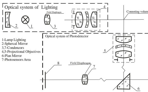
Figure 1: Optical scheme of OEU aerosol spectrometer “Masnik-A”.
