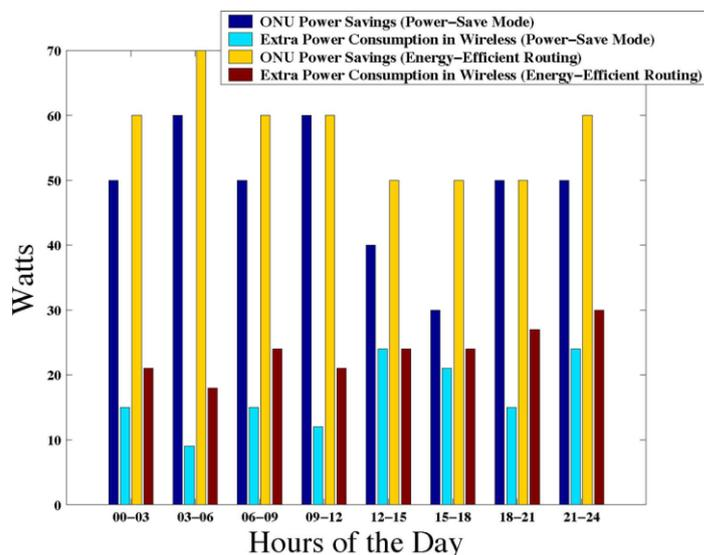
Fig. 4. Power savings versus extra wireless power.
