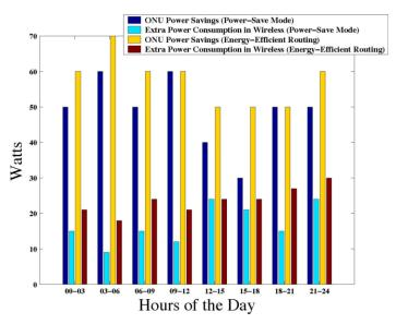
Fig. 4 .Power savings versus extra wireless power.
